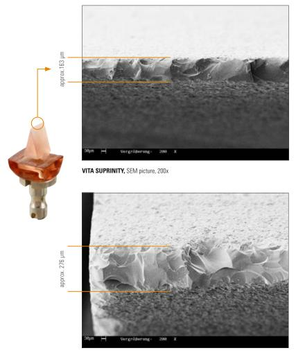
Lithium disilicate ceramic, SEM picture, 200 x
